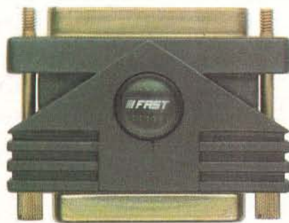
Hardlock E-Y-E – custom chip for software protection.
